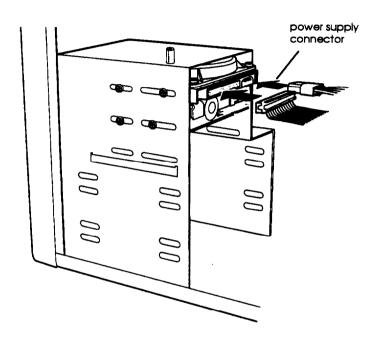
9. Locate one of the cables that lead from the power supply. (They have multi-colored wires and a plastic connector on the end.) Align the notched comers of the power supply connector and the drive's power connector; then push in the connector.
